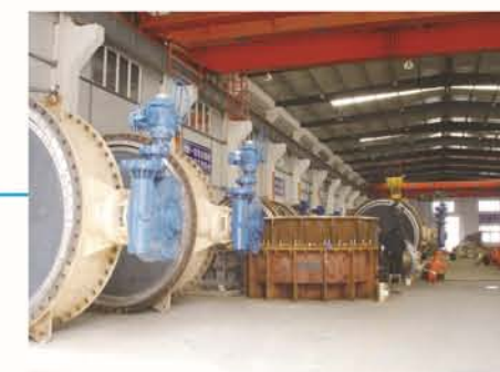
Butterfly Valve Assembling workshop
